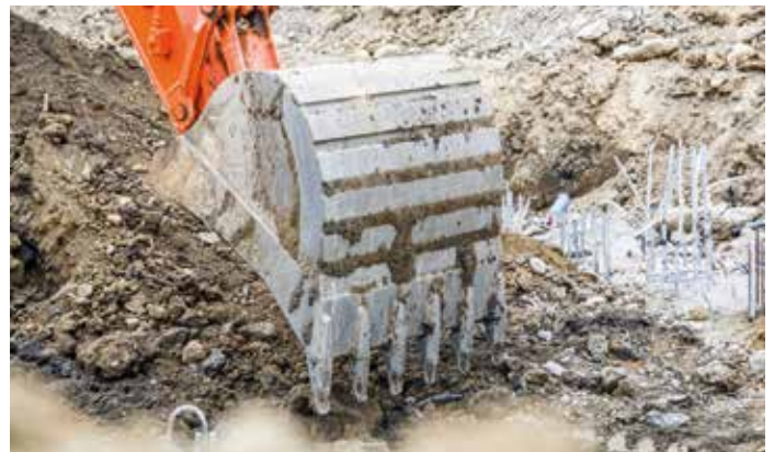
Hitachi GET include self-sharpening teeth and reliable adapters to ensure a precise fit.
